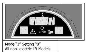
To adjust Programming mode depress light switch, whilst in calibration mode.
