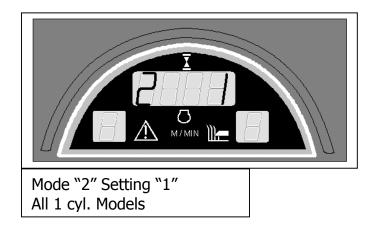
To change display numbers when calibrating, use the light switch to change the calibration mode & the electric clutch switch to change the setting. The programming **must** be done in sequence. I.e. Mode 1, Mode 2 etc. Once the settings have been made turn the ignition switch off to save the calibration.
