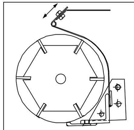
to take the mower to an authorized service agent for checking over and possible modification to the grass thrower plate.
