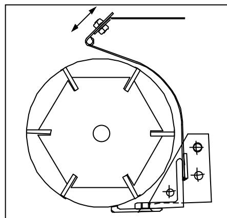
**Catcher:** Check the grass catcher frequently for wear or deterioration.
