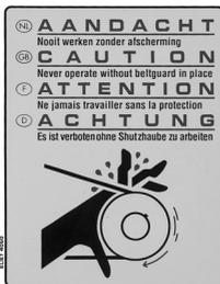
This sticker is attached to the drive belt guard. The sticker points out the danger which can occur if the guard is removed while the motor is rotating. Never operate the machine if the guard is not in place.
