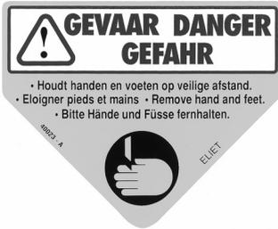
This sticker is attached to the safety net and warns against the danger of injury to hands. The screen on the shredding chamber should only be opened once the knives have come to a complete standstill. The motor should always be switched off before lifting the safety net.
