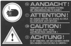
This sticker is attached in the input opening. The sticker emphatically points out the risk of injury to hands which is inherent in wood shredding. The sticker reminds the operator how to operate the shredder in the safest possible way. It is prohibited to insert your hands beyond the safety shield!
