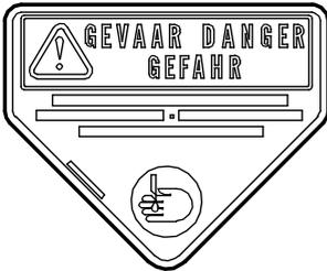
This sticker is affixed on the belt protection cover and warns about the danger of hand injuries. Keep your hands and feet away from underneath the machine as long as the blades are rotating. The engine must be turned off in case of faulty operation or before starting maintenance.
