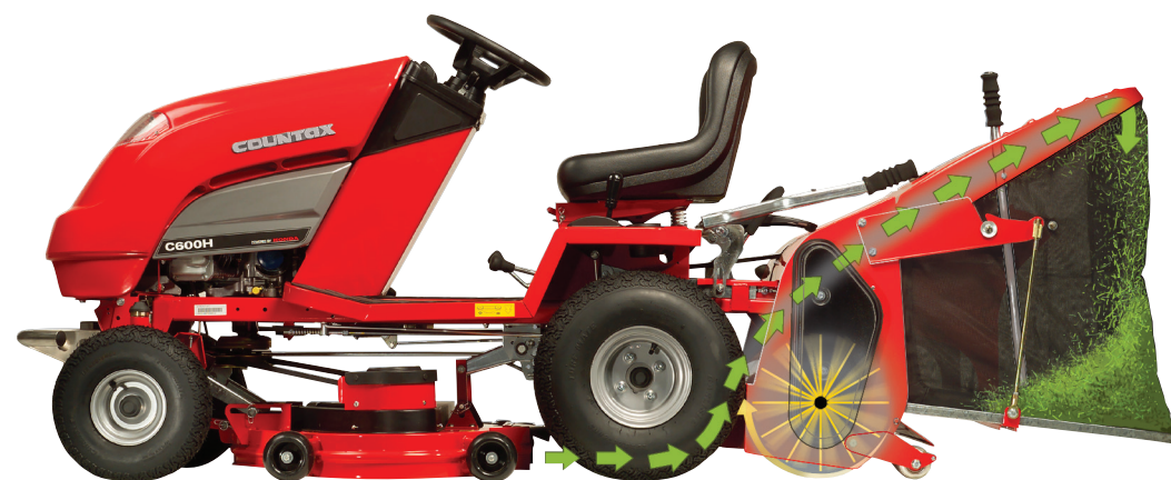
Brushes rotate against the forward motion of the tractor, throwing clippings to the rear of the collector's hopper.
