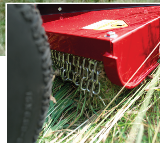
Grass and weeds are trapped in the High Grass Mulching deck while tough blades cut and reduce them to a mulch.
