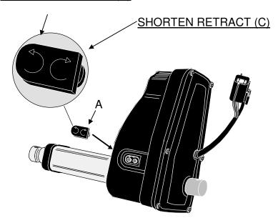
If the adjustment screws have been incorrectly adjusted the actuator may stall at the end stroke and/or blow a fuse.
